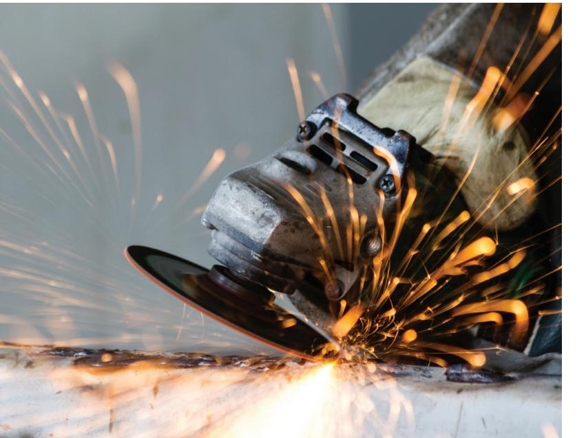
Prior to abrasive blasting and subsequent coating application, it is important to address surface defects in structural steel and other metallic substrates such as rough welds, weld spatter, flame cut edges, laminations, protrusions, and sharp edges. NACE SP-0178 may be used as a guideline for specifying the degree of mechanical surface preparation required.
